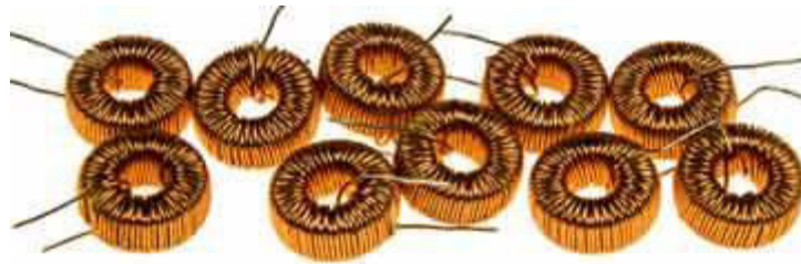
Inductors on a toroidal ferrite former
